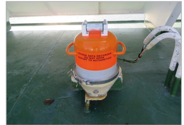
Figure 12: The protective capsule (or final recording media) of a voyage data recorder on M/V Barfleuer. (Edward Betts, Wikimedia)
