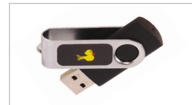
Figure 9 A $50 covert USB device that is designed to be quickly connected to a computer and used to inject keystrokes to download malware for remote access.
